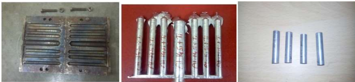
Fig.2.Preparation of Al-Si Alloys (a) Graphite mould, (b) Alloys after casting, (c) Specimens used for wear test
